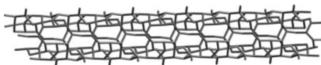
Figure 3. The generation of a water pipe formed by the repetition of (\text{H}_2\text{O})_{13} cluster (as shown in Figure 2).
